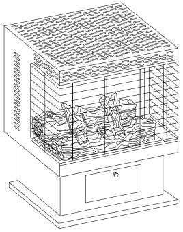
FIGURE 1.9830 Vent-Free Pedestal Gas Heater.
